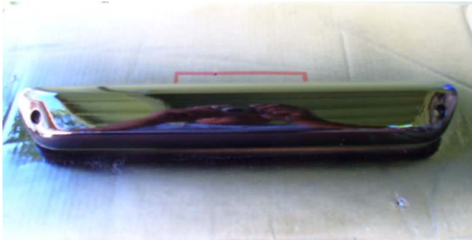
Figure 2: After the wet clear coats
